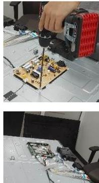
LCD (together with their casing) is only left after all other parts like electronic units have been removed.
