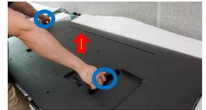
Once removed, this will expose the accessible electronic units (PCBs) which can now be easily removed with hand and screw driver.
